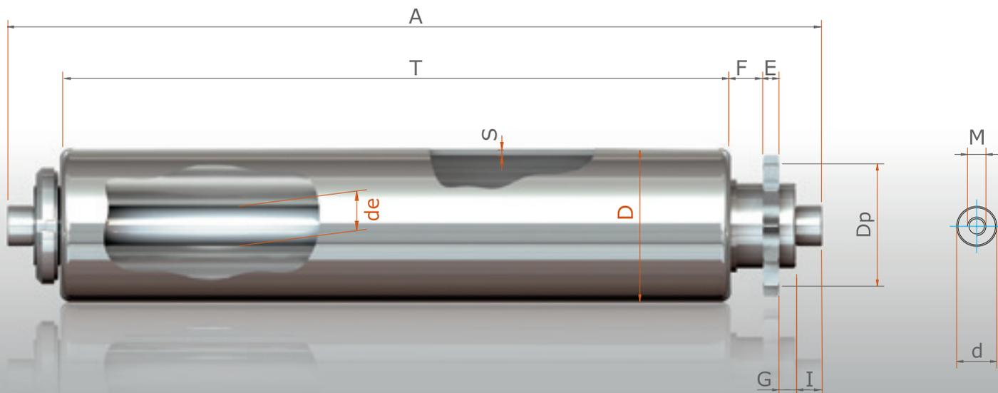
**RULLI CON DOPPIA FRIZIONE PFS2 - PFA2 ADJUSTABLE DOUBLE FRICTION ROLLERS**
